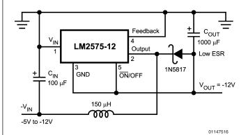
Typical Load Current 200 mA for  $V_{IN} = -5.2V$
