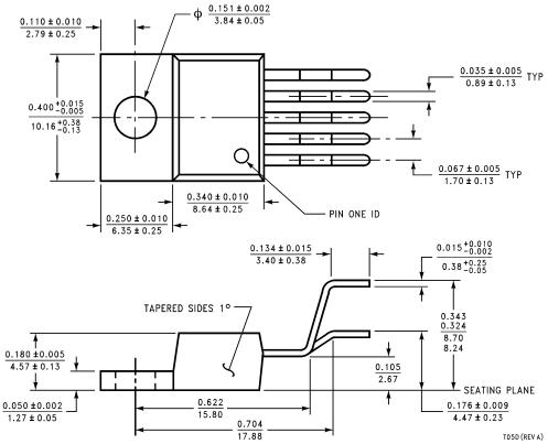
Bent, Staggered 5-Lead TO-220 (T)
