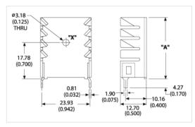
X Dim: 11.18 (0.440) | Y Dim: 8.26 (0.325) | Z Dim: 2.39 (0.094)
