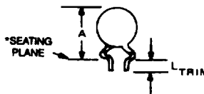
*Seating plane interpretation per IEC-717 CRIMPED AND TRIMMED LEAD
