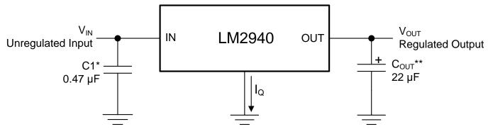
\*Required if regulator is located far from power supply filter. \*\*C<sub>OUT</sub> must be at least 22 µF to maintain stability. May be increased without bound to maintain regulation during transients. Locate as close as possible to the regulator. This capacitor must be rated over the same operating temperature range as the regulator and the ESR is critical; see curve.
