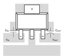
Figure 31. LM2940 SOT-223 Layout
