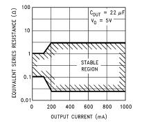
Figure 27. Output Capacitor ESR Limits
