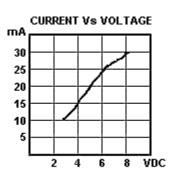
\*\*Note - Frequency is 2.8 KHz. + 0.2 KHz. from 3 to 8 VDC
