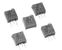
The Model 64 is a small size trimmer -  $3/8" \times 3/8" \times 3/16"$  answering PC board mounting requirements. Five versions are available which differ by the position of the control screw in relation to the PC board plane and by the spacing of the terminals. Excellent operational stability is provided by the use of a cermet element.
