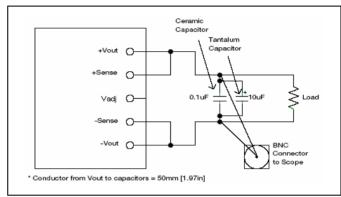
Output ripple and noise test setup
