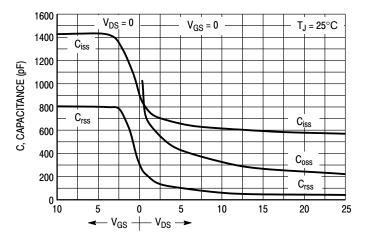
GATE-TO-SOURCE OR DRAIN-TO-SOURCE VOLTAGE (VOLTS)
