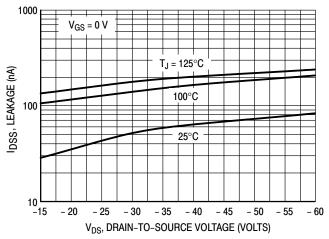
Figure 6. Drain-To-Source Leakage Current versus Voltage
