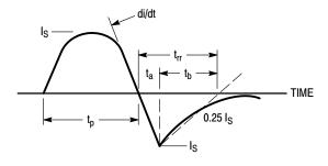
Figure 14. Diode Reverse Recovery Waveform
