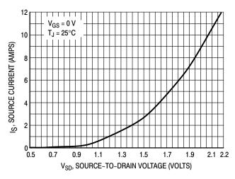
Figure 10. Diode Forward Voltage versus Current
