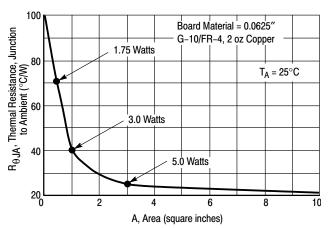
Figure 15. Thermal Resistance versus Drain Pad Area for the DPAK Package (Typical)
