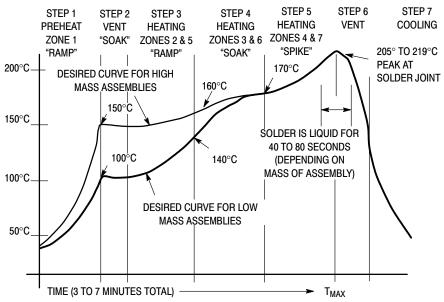
Figure 17. Typical Solder Heating Profile
