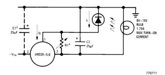
\*Lamp brightness increases until  $i_1 = i_Q (1 \text{ mA}) + 5V/R1.$ †Necessary only if raw supply filter capacitor is more than 2 inches from LM320.
