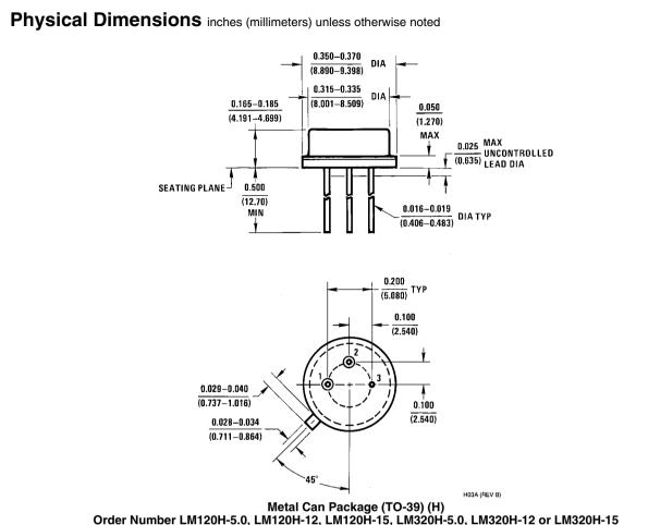
Metal Can Package (TO-39) (H) Order Number LM120H-5.0, LM120H-12, LM120H-15, LM320H-5.0, LM320H-12 or LM320H-15 NS Package Number H03A
