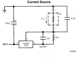
$$*I_{OUT} = 1 \text{ mA} + \frac{5.0 \text{V}}{\text{R1}}$$
