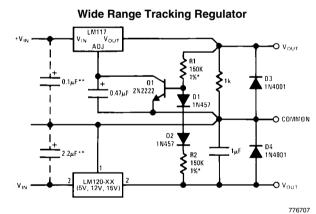
\*Resistor tolerance of R1 and R2 determine matching of (+) and (-) inputs. \*\*Necessary only if raw supply capacitors are more than 3 from regulators An LM3086N array may substitute for Q1, D1 and D2 for better stability and tracking. In the array diode transistors Q5 and Q4 (in parallel) make up D2; similarly, Q1 and Q2 become D1 and Q3 replaces the 2N2222.
