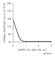
FIGURE 6.  $\theta_{\rm (J-A)}$  vs Copper (2 ounce) Area for the SOT-223 Package
