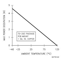
FIGURE 5. Maximum Power Dissipation vs  $T_{\rm AMB}$  for the TO-263 Package
