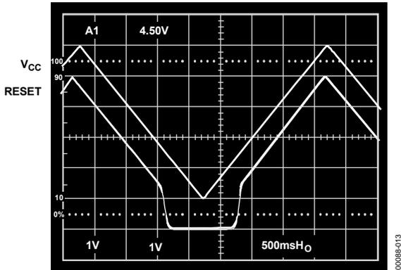
Figure 7. ADM707/ADM708  $\overline{\text{RESET}}$  Output Voltage vs. Supply Voltage
