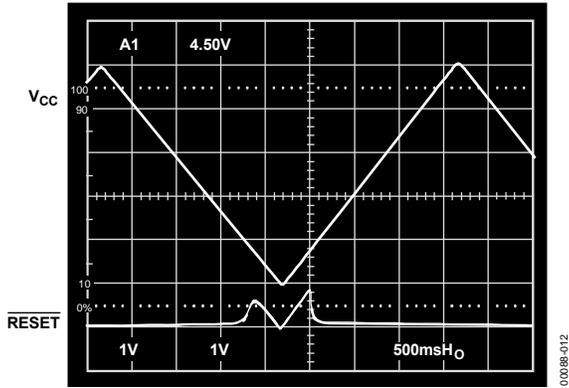
Figure 6.  $\overline{\text{RESET}}$  Output Voltage vs. Supply Voltage
