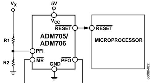
Figure 20. Monitoring 5V and an Additional Supply,  $V_x$
