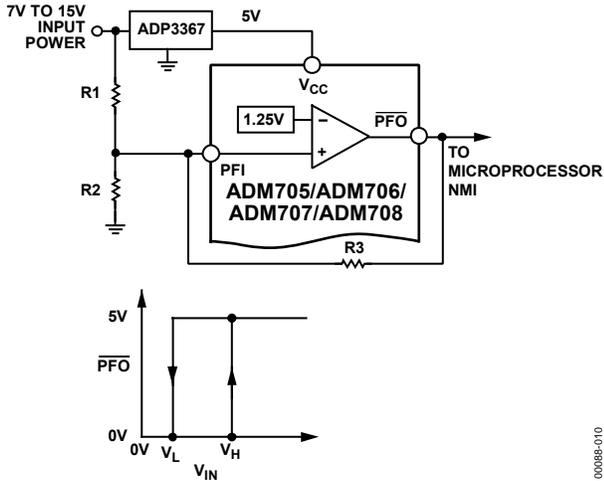
Figure 16. Adding Hysteresis to the Power-Fail Comparator
