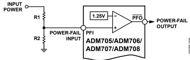
Figure 15. Power-Fail Comparator
