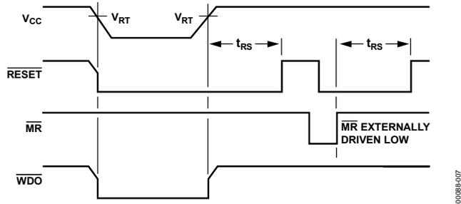
Figure 13.  $\overline{\text{RESET}}$ ,  $\overline{\text{MR}}$ , and  $\overline{\text{WDO}}$  Timing
